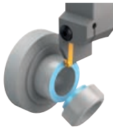
Neutral cutting insert: Burr on the right of the tube
