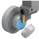
Neutral cutting insert: Pips on the workpiece
