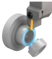
Neutral cutting insert: Burr on the right of the pipe
