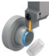
Left-hand cutting insert: Burr on the left of the pipe
