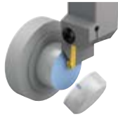
Neutral cutting insert: Pips on the workpiece
