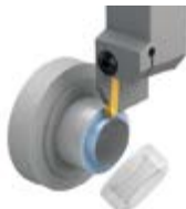
Left-hand cutting insert: Burr on the left of the tube
