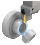
Neutral cutting insert: Burr on the right of the tube
