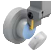
Right-hand cutting insert: Pips on the workpiece
